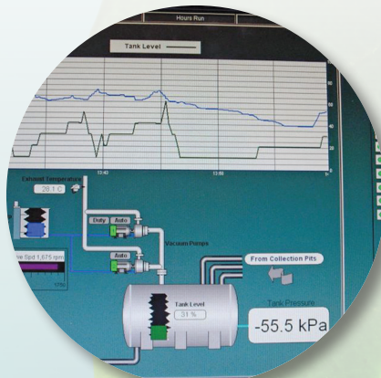
Monitor the Electrical and Mechanical Equipment at the Vacuum Pump Station
